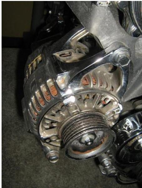
Figure 70 Alternator on a car (Image by Christopher Ziemnowicz, Wikimedia Commons)
